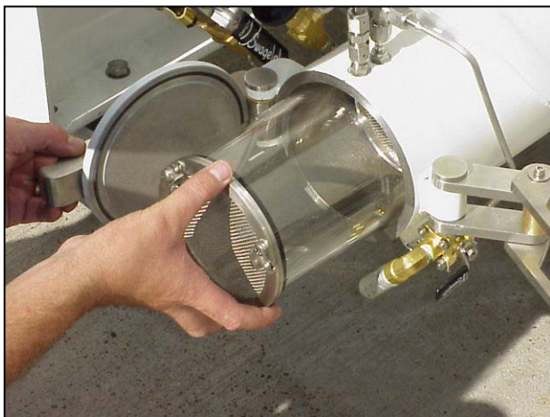
CO2 Scrubber canister removed through Medical Lock
